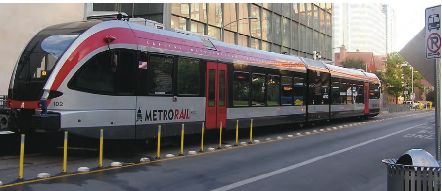
Light DMUs get 2 mpg for 160 seats, vs. 1 mpg for SMART trains, and can operate "in street" over 1-2 miles. Wikipedia. By Michlaovic - Own work, Public Domain
