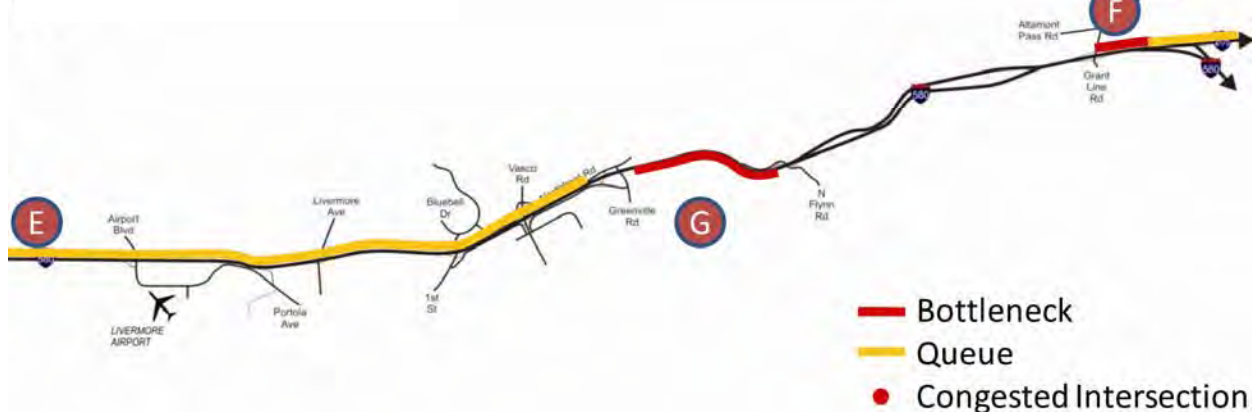
Figure 5: Existing 2008 Recurrent Weekday Congestion on I-580 (from ALA-238/580 Corridor System Management Plan Technical Analysis Report-Volume 1, Section 2, Figure 21, page 69)
