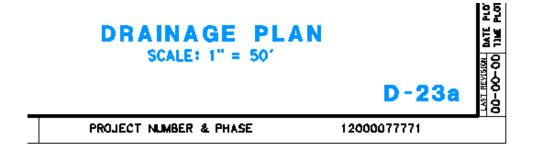
Note: A <u>lowercase</u> letter is used in the name of the MicroStation design file, TIFF file, Sheet ID and the sheet numbers in the Project Identification Block when revised or additional sheet are added to the As-Built plans. During the addendum process (which is prior to contract award), an <u>uppercase</u> letter is used in the Sheet ID when a sheet is added (see the Ready To List and Construction Contract Award Guide - RTL Guide).
