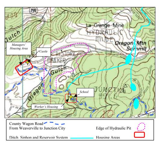
Map 3 shows the La Grange Hydraulic Mining complex and the topography of the site. The closer the lines are to one another, the steeper the terrain. The map also shows the location of the ditch, siphon, and reservoir system that supplied the mine with water.
