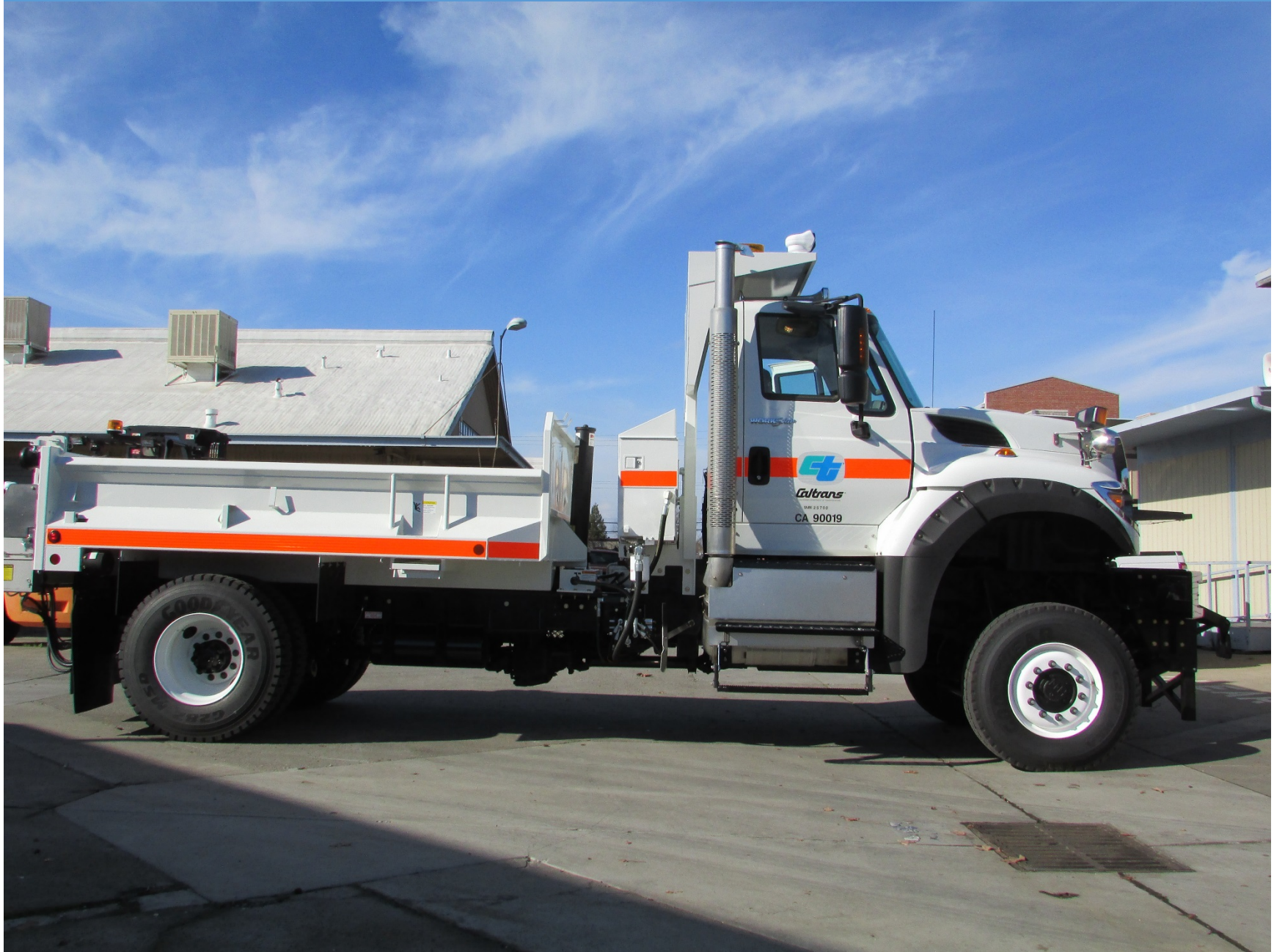
MAINTENANCE CLASS 13724 DUMP BODY, 4 CY, 4x4, W PUSH PLOW & SPREADER, DSL
