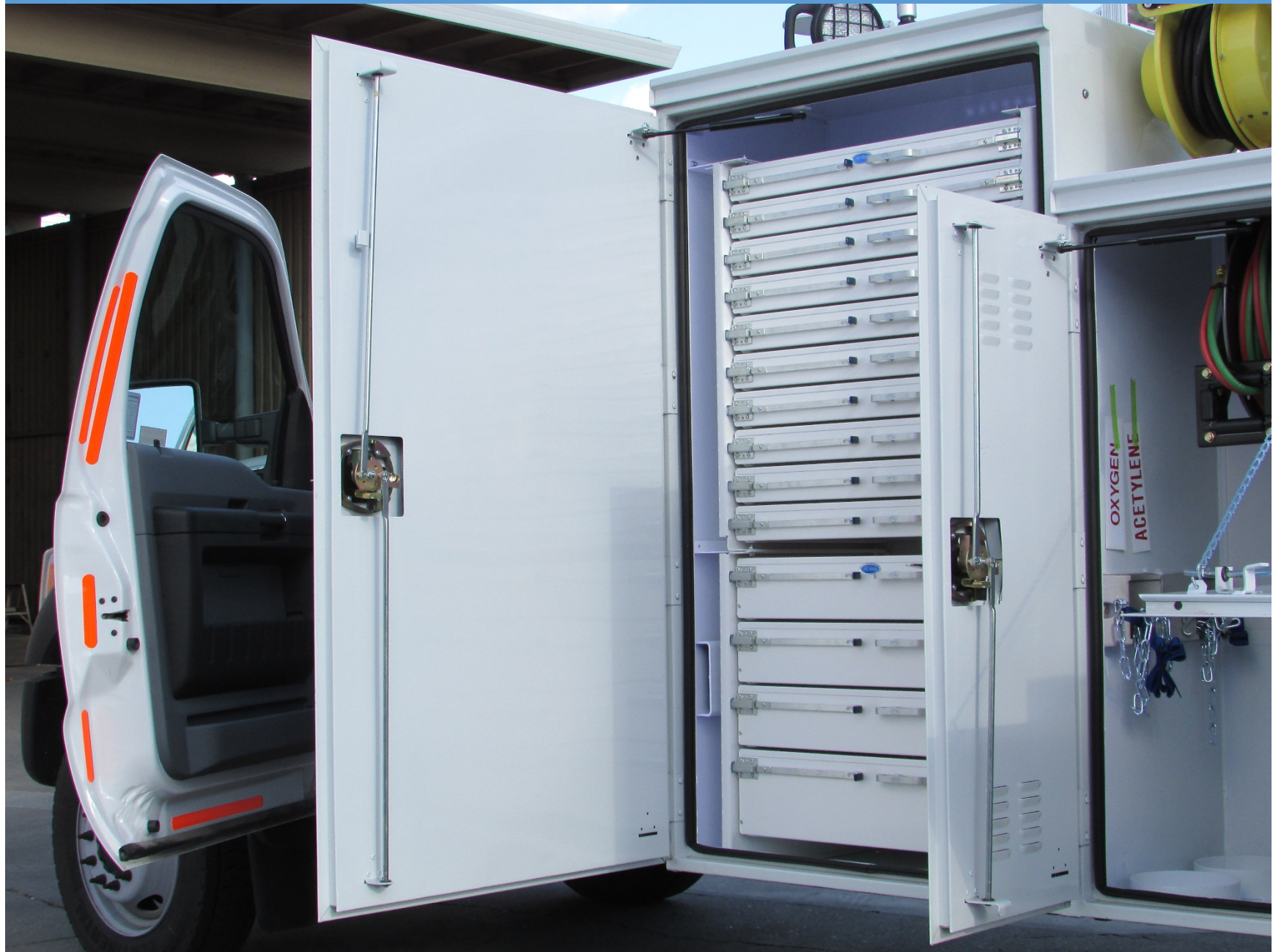
MAINTENANCE CLASS 01436 MECHANIC BODY, 1-TON, SUPER DUTY, GAS
