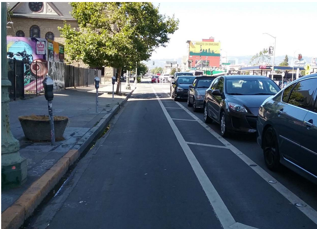
Photo 4: Separated Bikeway with parking in Oakland
