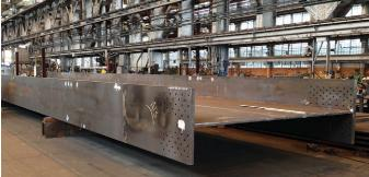
Crews demolished the Pfeiffer Canyon Bridge in March following torrential rains in February that damaged the span. Its replacement is expected to open in mid to late September, using 15 steel girders being constructed in Vallejo, bottom right. Each girder is 63 feet long and weighs 56 tons. They will be connected on site, then rolled into place across the canyon using strategically placed winches and cables.
