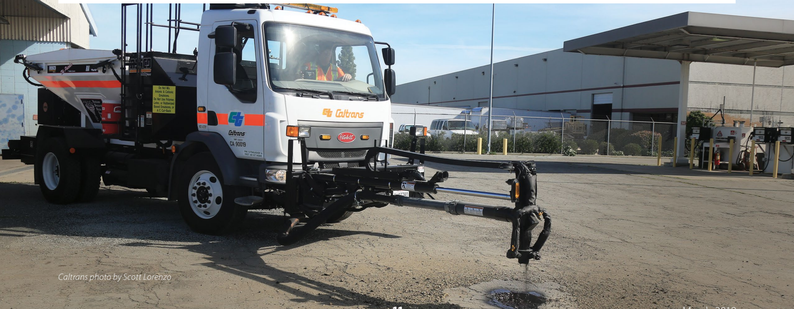
Below, a pothole patcher mounted on a truck body. Because it is motorized, the patcher reduces the need for workers on a busy roadway, and fewer full-lane closures are required for maintenance activities. Repairing potholes is among the leading service requests submitted by the public.
