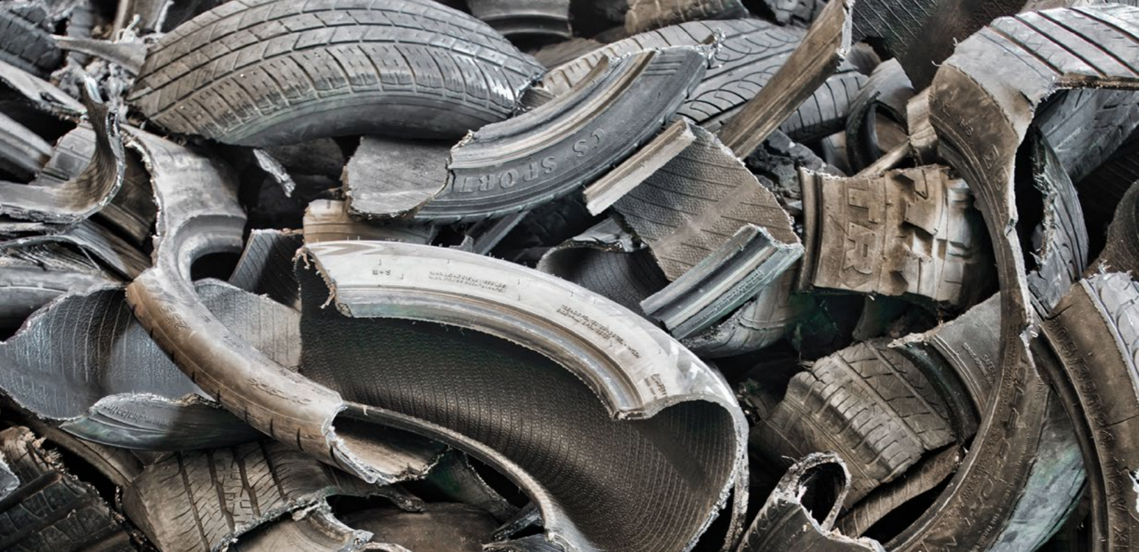
These unsightly hunks of waste tires await further processing into crumb rubber, the particles of which are blended with asphalt paving mixes for use in Caltrans maintenance and construction projects. Caltrans asphalt mixes contained an average of almost 40 percent crumb rubber in 2016.
