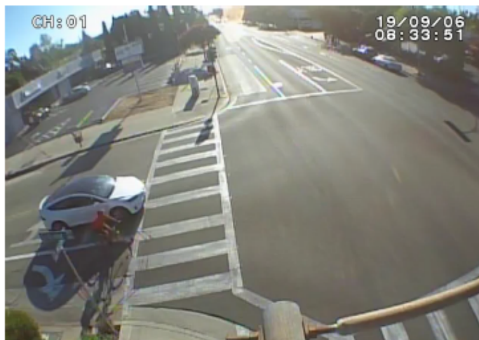
When a car covers the bike box, bicyclists sometimes choose to wait on the right side of the vehicle.
