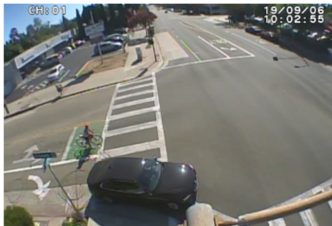
A bicyclist who stops on a through-lane bike box allows cars in the right-turn lane to turn right on red, as shown here at Grand Avenue & Mission Street after bike box installation.
