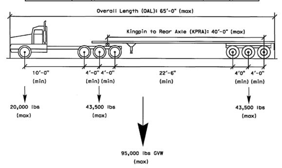
Figure 202.2 Overweight Intermodal Cargo Container Permit Vehicle – Allowable Axle and Gross Vehicle Weights
