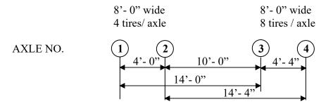
In the above example axles 1 & 2 have a "Bonus Factor" of 1.0 for each axle. Axles 3 & 4 have a "Bonus Factor" of 1.15 for each axle.
