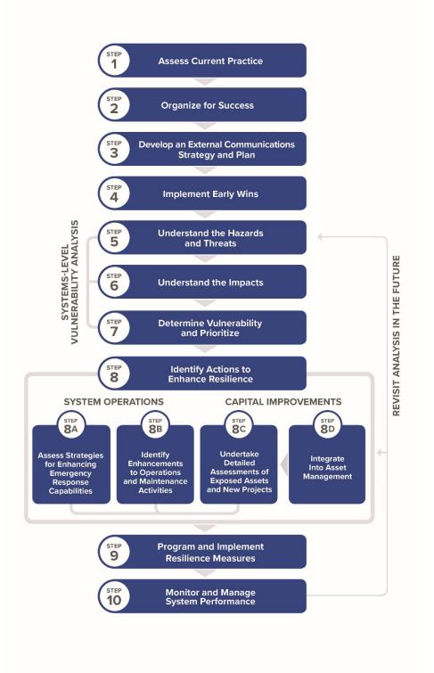
FIGURE 1: CALTRANS' CLIMATE ADAPTATION FRAMEWORK (FEAR-NAHT FRAMEWORK)
