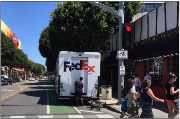
Figure J.4. Curbside Bicycle Lane Complicates Truck Access to the Curb
