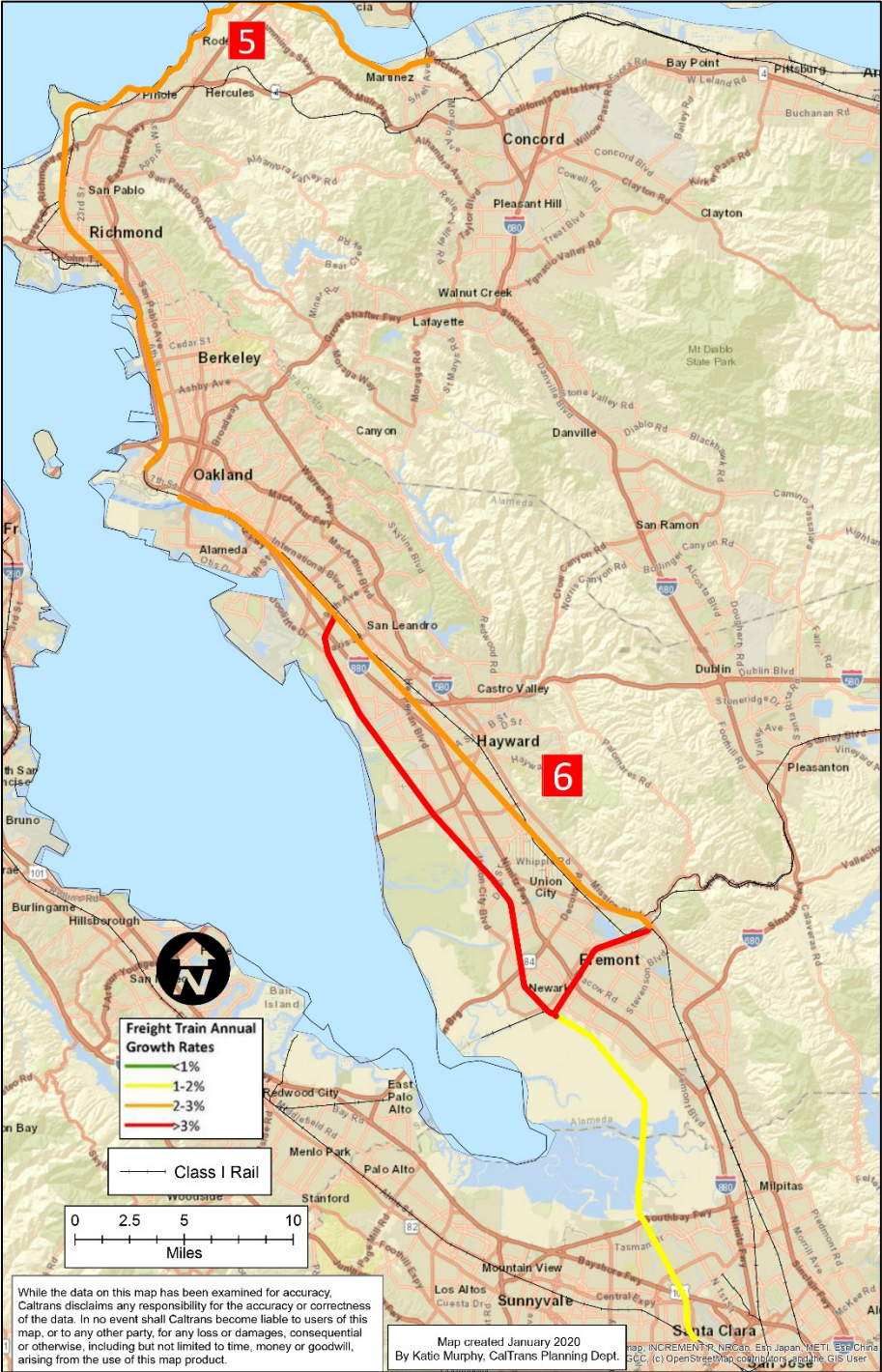
Figure 3B.5.2. Heavy Rail Freight Traffic Corridor Bottlenecks in Northern California – Segments 5 and 6
