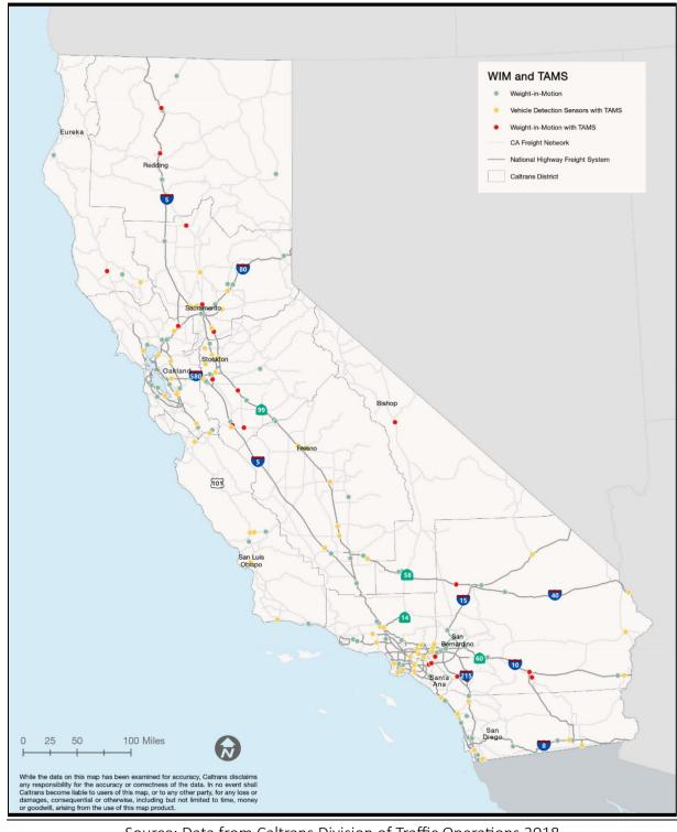
Figure 3A.7. California Weigh-In-Motion Stations and Truck Activity Monitoring Stations
